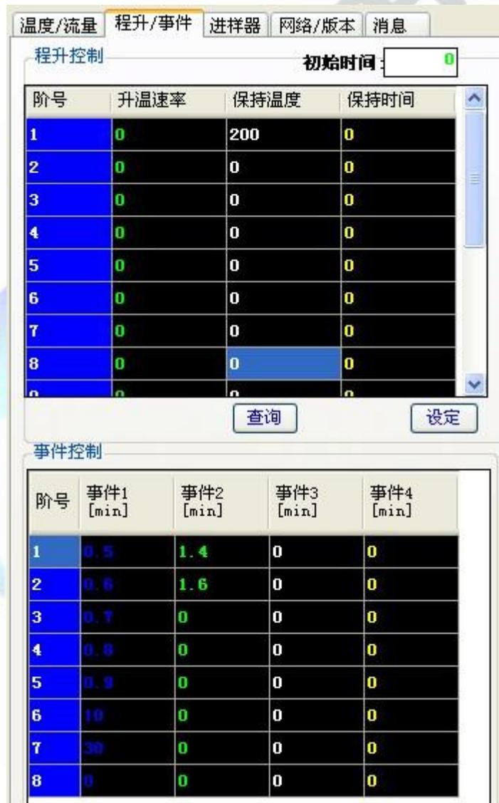
The screenshot shows a software interface with two main sections: "程升控制" (Program Temperature Control) and "事件控制" (Event Control). The "程升控制" section includes a table with columns for "阶号" (Step No.), "升温速率" (Ramp Rate), "保持温度" (Hold Temperature), and "保持时间" (Hold Time). The "事件控制" section includes a table with columns for "阶号" (Step No.) and four event time points: "事件1 [min]", "事件2 [min]", "事件3 [min]", and "事件4 [min]".
